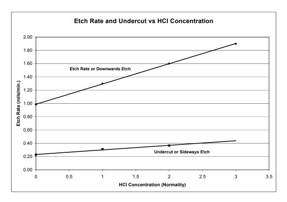
Unfortunately, as also shown on the graph, increasing the acid concentration also increases the rate of undercut or lateral etch. The rate of undercut almost doubles
