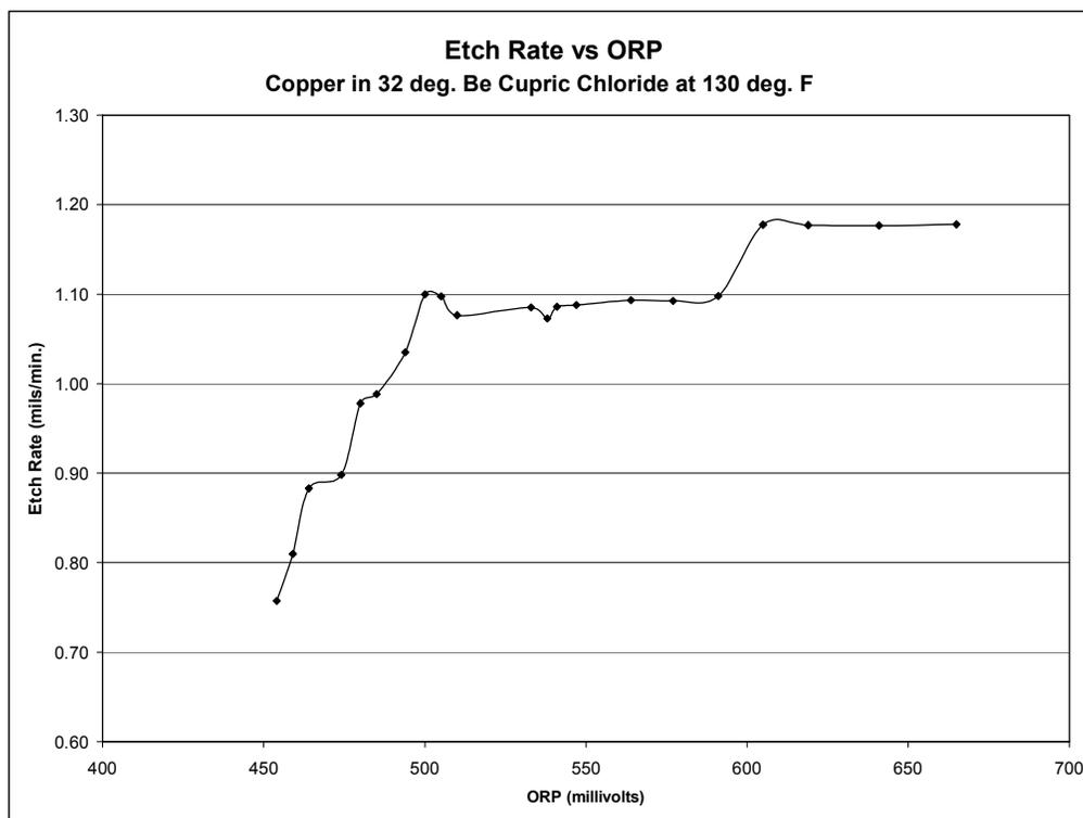
The etch rate of cupric chloride changes fairly rapidly as the ORP changes except for the region between 500 mv and 600 mv where the etch rate remains fairly steady. Since this plateau occurs at a fairly high etch rate it provides an excellent range to use as a control setting. Setting the ORP controller to the midpoint of this
